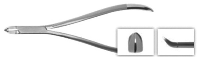
66-5181 Mini or Normal Handled Ligature Cutter Upper Standard Handle The narrow tip is angled at 50 for excellent access to the upper arch. Minimum Cutting Capacity: soft wire up to .012" (.30mm)
