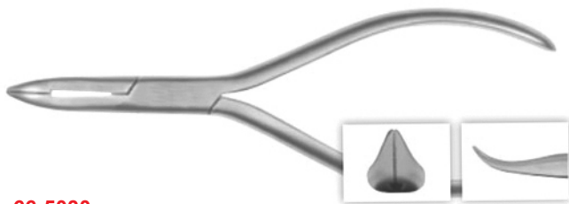
66-5030 Fine Tipped Weingart Sturdy construction without T.C. This strong but fine tipped utility plier allows excellent access in difficult to reach area. Holds. Wire up to .022" x .028" (.56 x .71mm)
