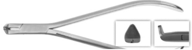
66-5177 Long Handle Distal End Cutter with TC Minimum Cutting Capacity: .014" (.30mm) Maximum Cutting Capacity: .019" x .025" (.48mm x .64mm) This instrument features long handles and a slim box joint with a compact head to ensure access in hard to reach areas.
