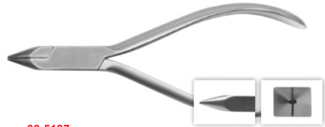
66-5137 Flat Nose Plier A favorite general plier - both tips of this flat nose plier are serrated with a guiding groove for use by technician or clinician for chairside adjustments of wire up to 0.7mm
